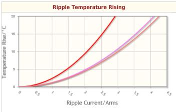
CGA4J3X7R1C475K125AB(100kHz) CGA4J3X7R1C475K125AB(500kHz) CGA4J3X7R1C475K125AB(1MHz)
